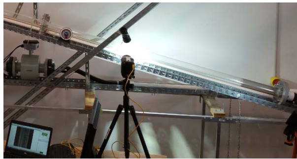
Figure 3.14 PTV system for measuring cuttings transport velocity.
