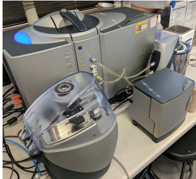
Figure 3.25 Malvern Mastersizer 3000 for wet cuttings size measurement.
