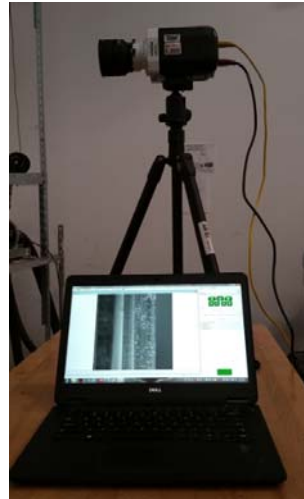
Figure 3.15 High speed camera and controlling computer.
