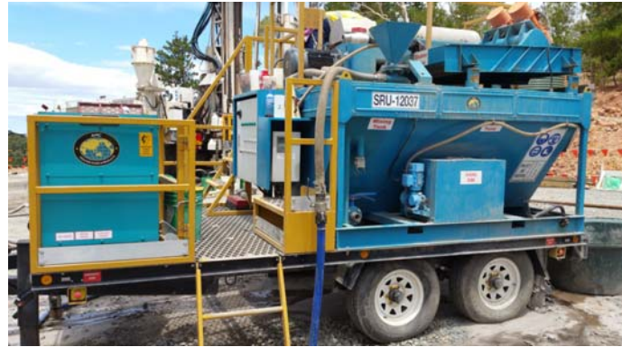
Figure 6.6 Solid removal unit (SRU) for drilling fluids circulation.
