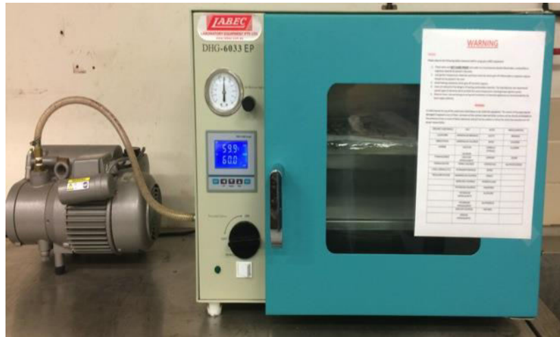
Figure 3.6 Vacuum oven LABEC DHG-6033EP.
