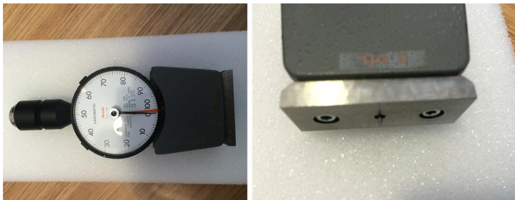
Figure 3.20 Mitutoyo analogue Durometer 811-337-01 hardmatic Shore type D
