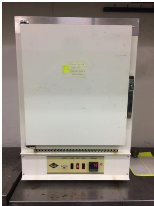
Figure 3.7 Circulating oven used in the curing process.
