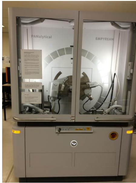
Figure 3.12 Picture of PANalytical EMPYREAN with a PIXcel 3D X-ray diffractometer.
