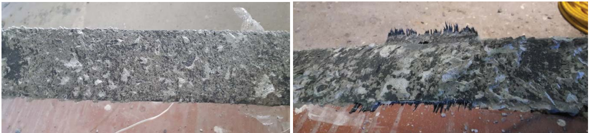
(b) Interfacial debonding in the shear span
