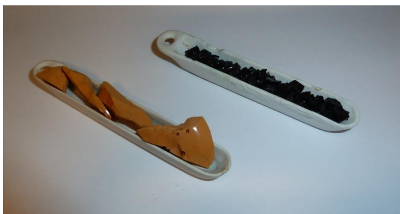
Figure 1.9 Illustration of resorcinol formaldehyde aerogel after curing (left) placed in a \text{Al}_2\text{O}_3 crucible and the pyrolyzed aerogel chopped into monolithic pieces of \sim 0.4 \text{ cm}^3 (right) which results in a graphite like structure. Photo credit: Payam Javadian.
