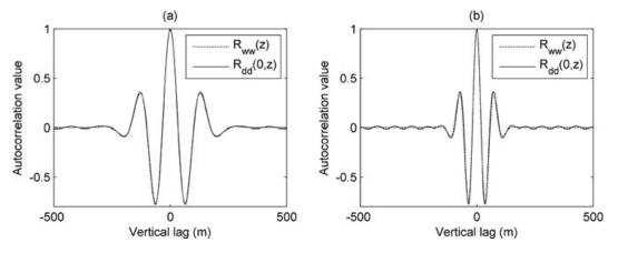
Figure 2. (a) Autocorrelation of the 15 Hz input wavelet used to create the FDTD data in Fig. 1(c) and vertical autocorrelation of the FDTD data. (b) Autocorrelation of the 27 Hz input wavelet used to create the FDTD data in Fig. 1(g) and vertical autocorrelation of the finite-difference modelled data.
