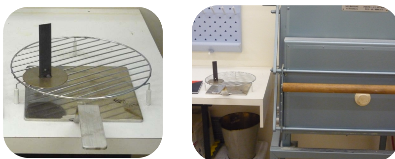
Figure 3.6. Vertical metal ruler on stand, wide flat lifter for puffed height measurement, and flat bread oven.
