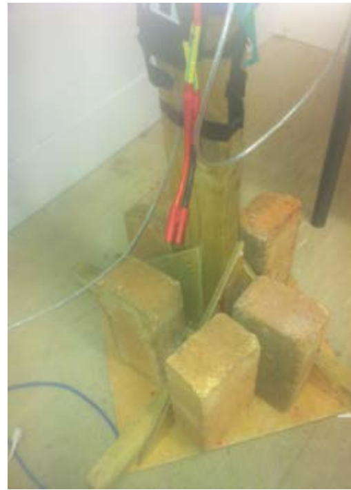
Figure 6-3: Quadrotor Test Stand Base.
