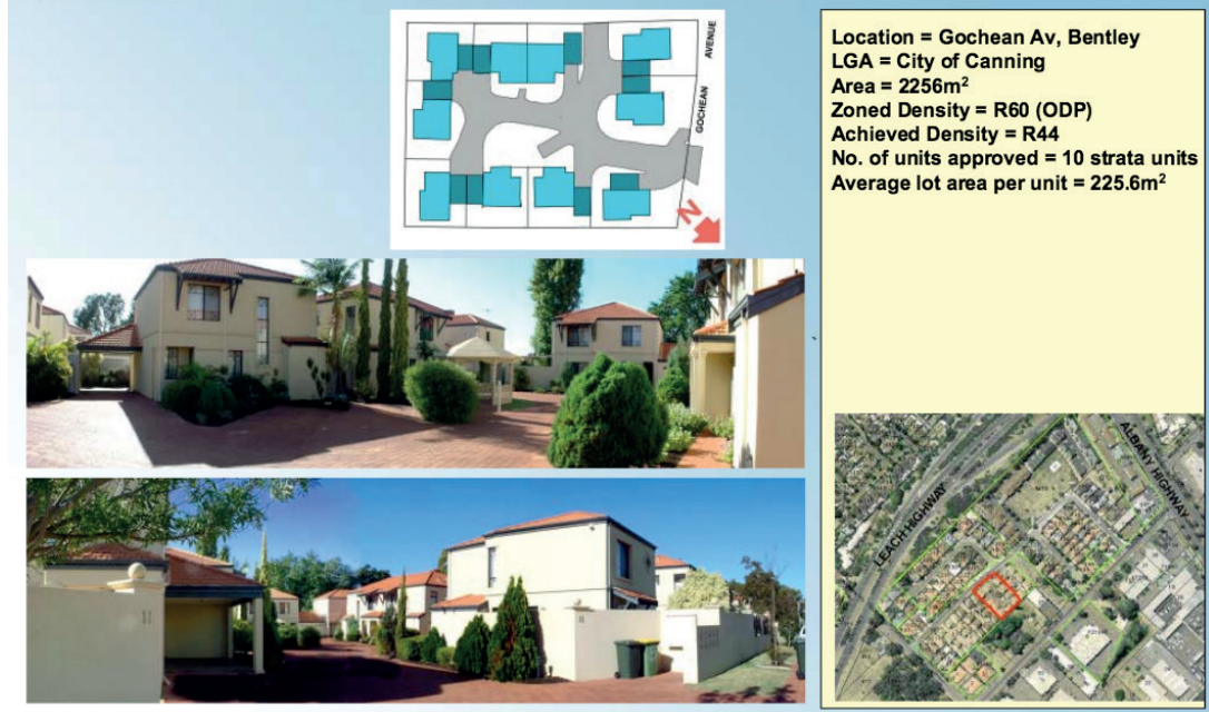
Figure 4: In Perth, the most typical infill is ‘deemed to comply’ under generic local planning controls but locks in suboptimal (auto-dependant) urban form.
