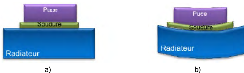
Fig. 4. 45. Electronic power device working in a) 25°C and b) 100°C
