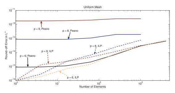
Figure 6: Round-off error for 2D Laplace problem discretized with uniform mesh.
