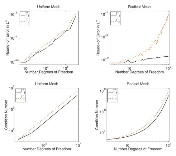
Figure 3: Log-Log representation of the condition number and round-off error for 1D Laplace problem discretized with a uniform grid (left) and a radical mesh (right). ILP shape functions of order p = 2 are used.
