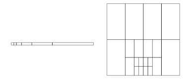
Figure 1: Left: Radical Mesh in 1D. Right: Radical Mesh in 2D.
