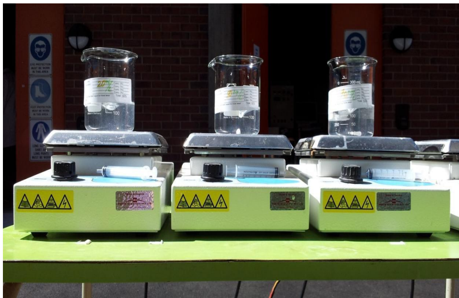
Figure 3.9 Photo Fenton experiment for oily wastewater treatment samples using natural solar light
