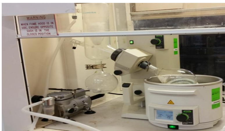
Figure 3.1 Rotary evaporator (Butchi Rotavapor) for oil content analysis
