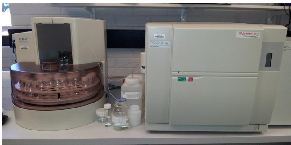
Figure 3.2 TOC analyzer for TOC measurement
