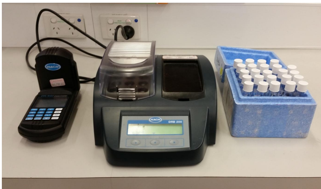
Figure 3.3 HACH DRB200 reactor and DR890 colorimeter for COD and Fe analysis
