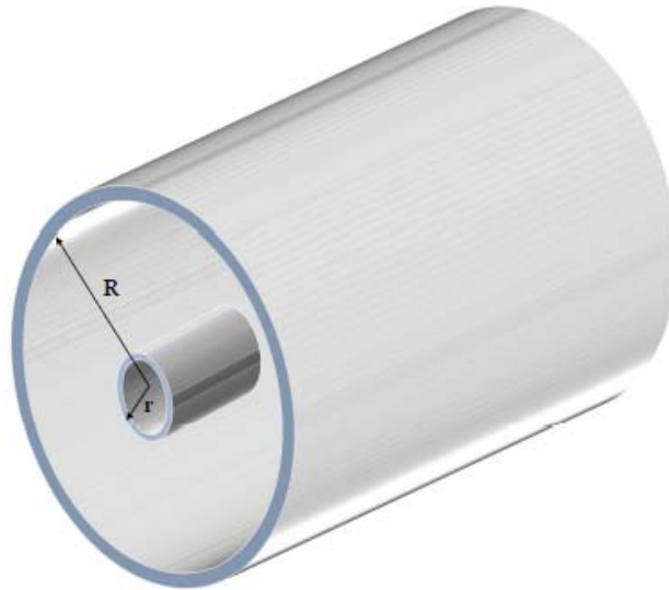
Fig. 3. 6 GIS bus duct cross section R: Inner diameter of GIS enclosure, r: Outside diameter of GIS bus duct
