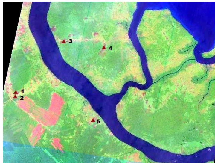
Figure 3.38. Detected FHS from the MODIS dataset of 20 Jan 2009 at 03:50 UTC using the MOD14 algorithm overlaid on the SPOT image for 22 Jan 2009 at 03:38 UTC (two days later); image block number K-J =272348
