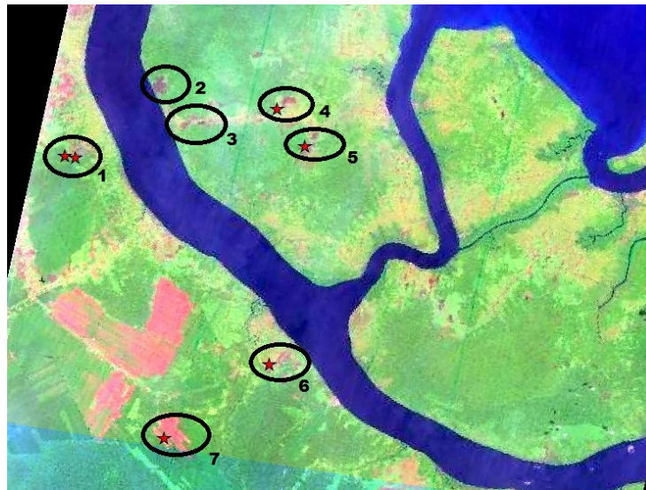
Figure 3.35. Detected FHS from MOD14 for 22 Jan 2009 at 03:40 UTC overlaid on a SPOT image for 22 Jan 2009 at 03:38 UTC; image block number K-J=272348
