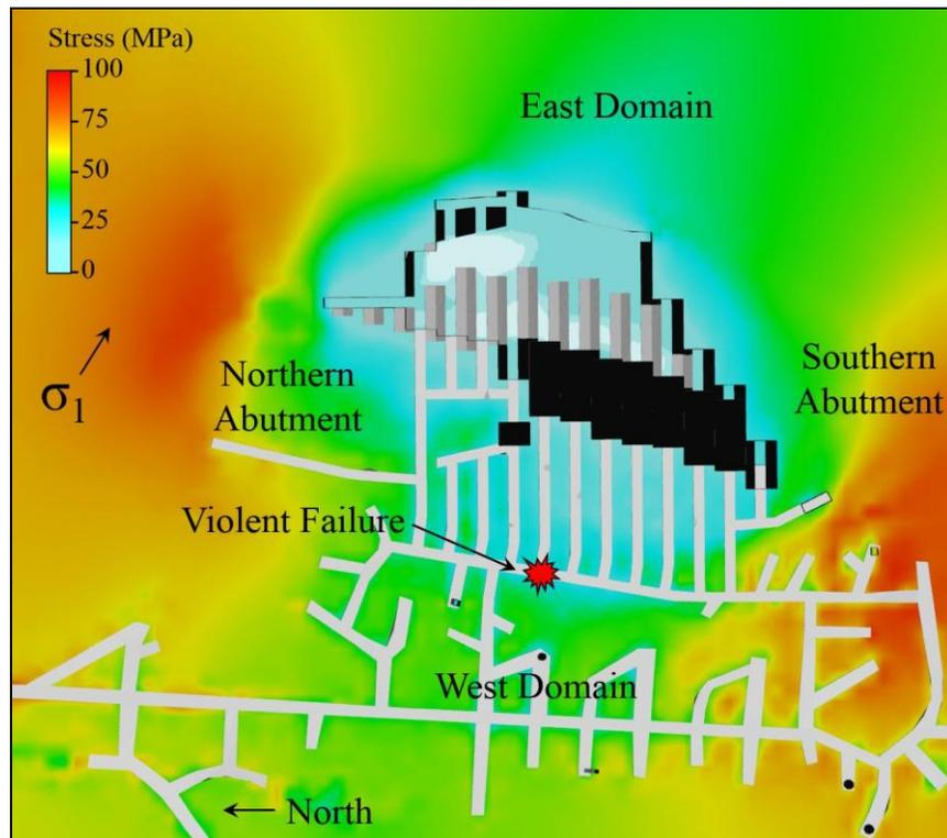
Figure 7 – Plan view of modelled mining induced stress around the cave at the time of violent failure, taken at a depth of 1055m.
