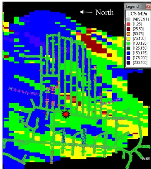
Figure 3 - UCS (MPa) block model for the mining level where violent failure occurred.
