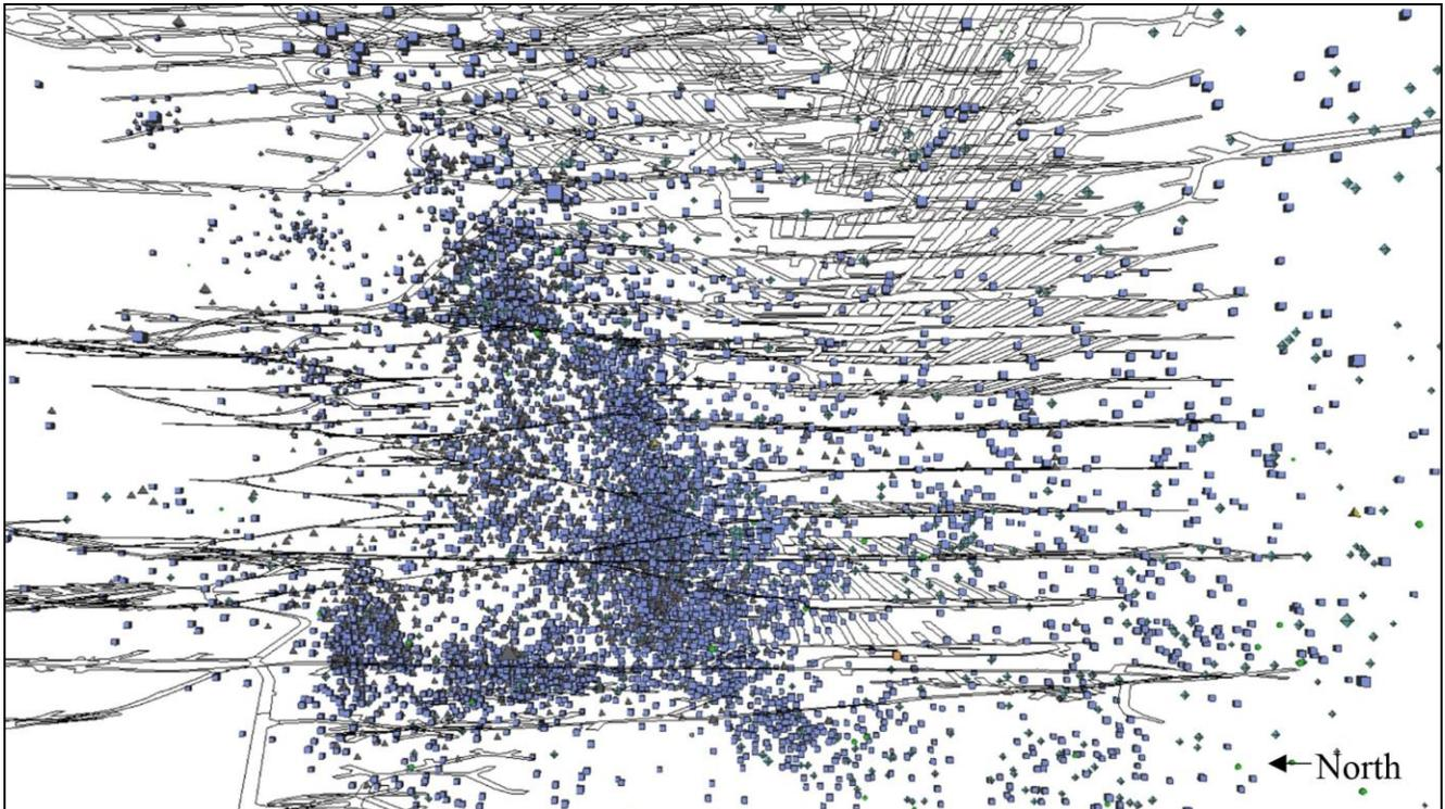
**Figure 8 - Seismogenic zone in the northern cave abutment following a large dynamic failure.**
