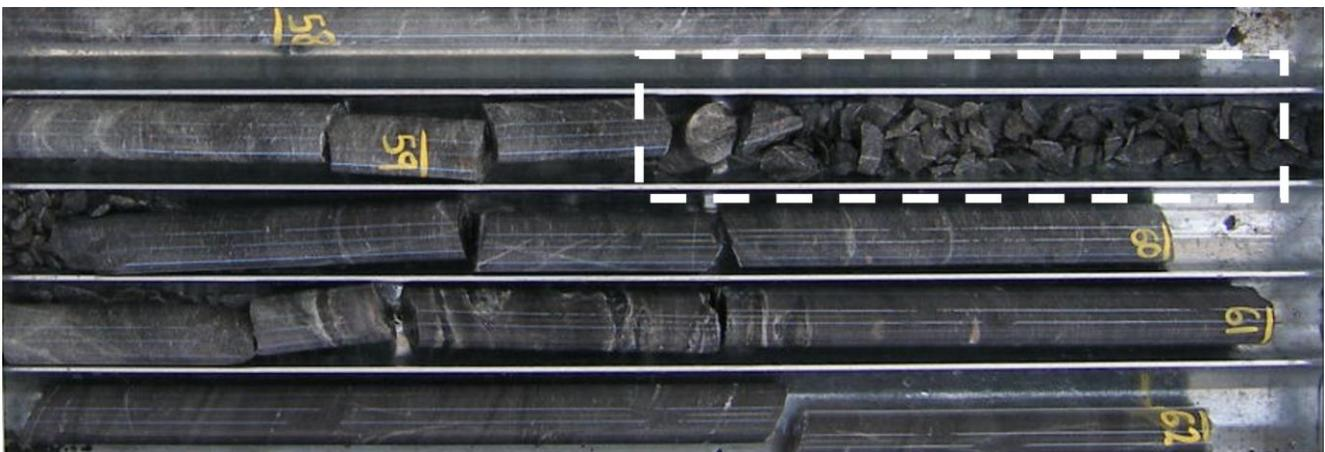
Figure 4 - Felsic drill core from the west domain showing intact rock and the effect of local geological structure.
