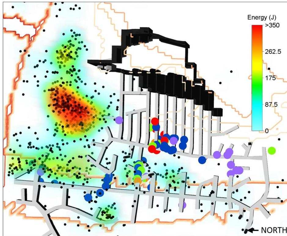
Figure 13 - Overlay of contours of radiated seismic energy, recorded seismic events and ground support damage locations.
