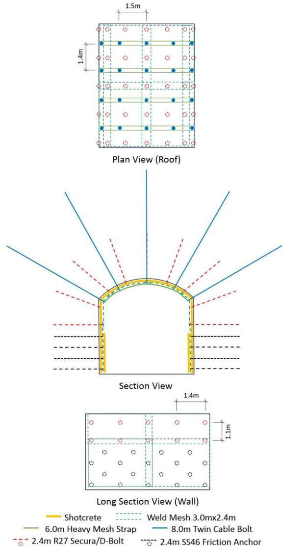
**Figure 11 - Second pass upgrade ground support scheme for deep development with 15-35kJ/m<sup>2</sup> demand. First pass ground support scheme is represented by dashed lines.**
