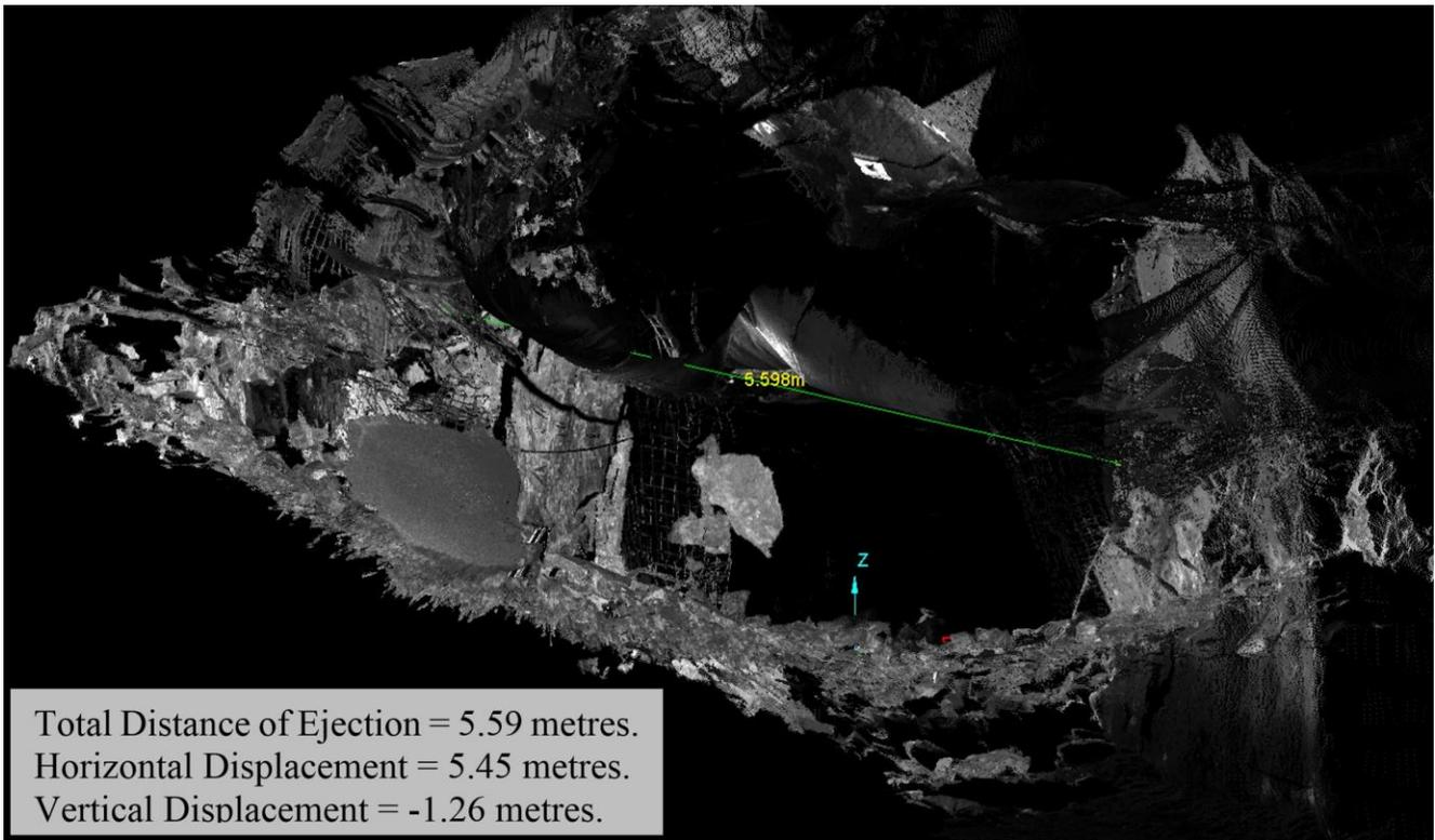
Figure 17 - Dimensions of the ejection path of the large block of support/rock, taken from HD survey scan data, view direction north, as in (Figure 14a).
