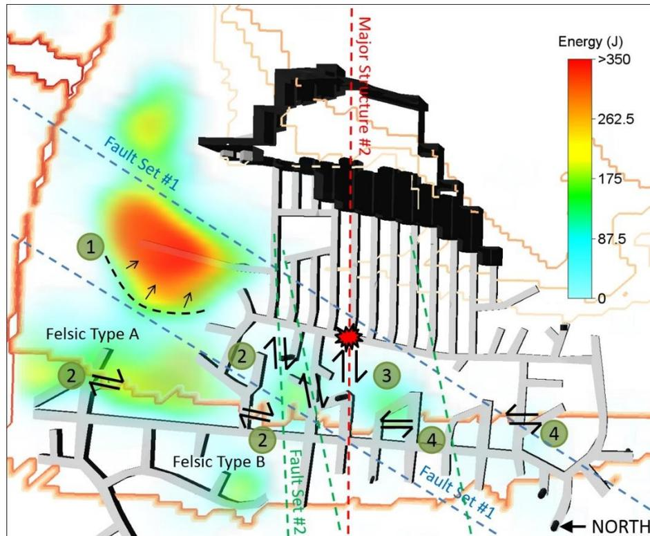
**Figure 12 - Failure mechanism sketch showing radiated seismic energy (inferred rock mass damage) and interpreted structural reactions.**
