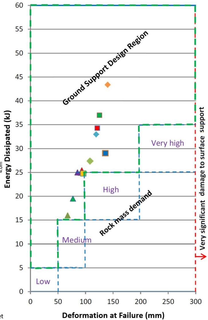
Figure 10 - Energy dissipated versus deformation at failure for combined schemes of rock bolts and mesh tested at WASM.
