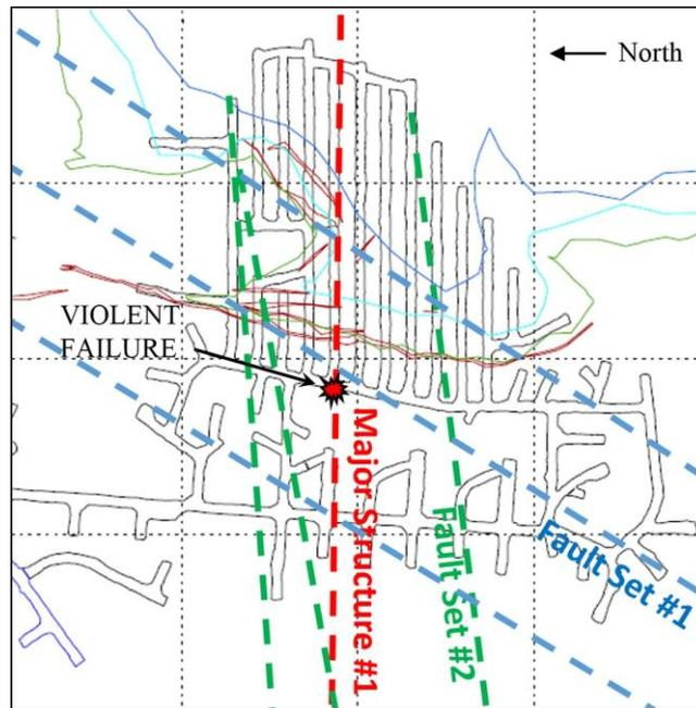
Figure 5 - Plan view sketch of mine development, basic geology and significant seismically active structures with respect to the location of violent failure.
