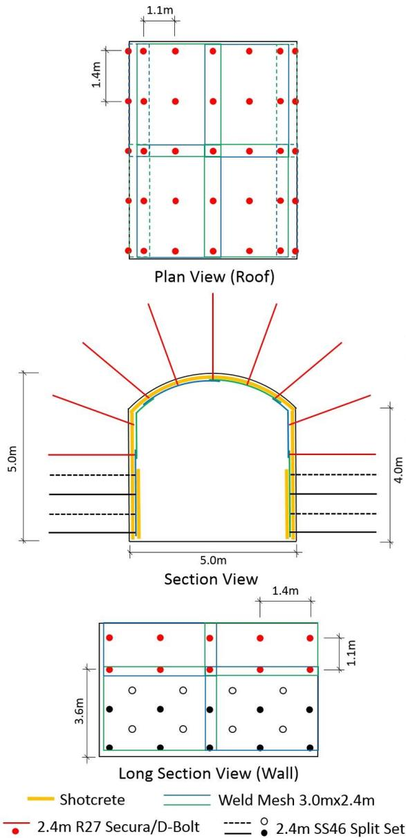
Figure 9 - Excavation shape and ground support scheme for conditions of medium energy demand.
