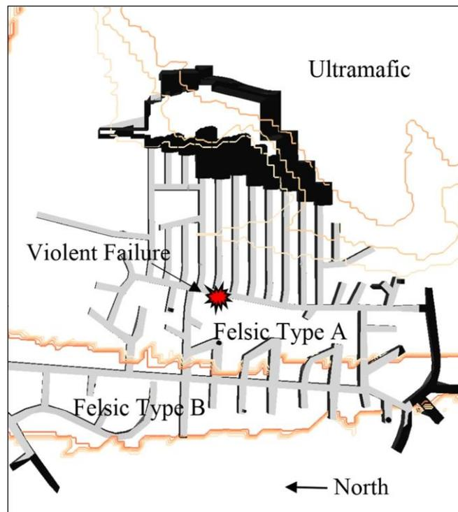
Figure 2 - Rock type boundaries where failure occurred.
