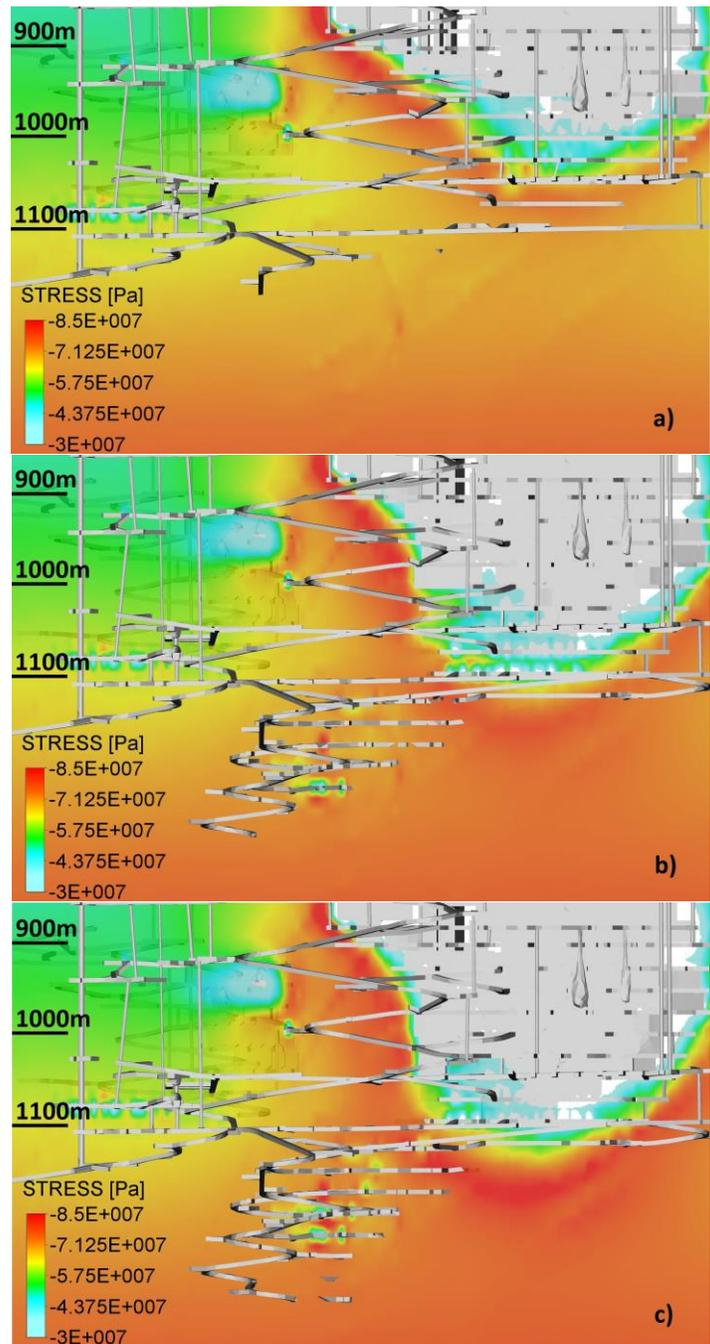
Figure 6 - Long sections of modelled major principal stress showing increasing stress concentrations in the cave abutments for three cave extraction steps.
