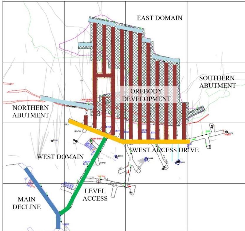
Figure 1 - Plan view of mining infrastructure (grid 100m).
