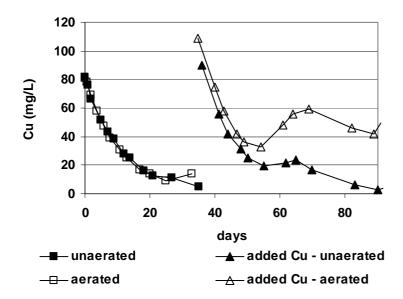
Figure 5. Copper concentrations in reservoir solutions for aerated and unaerated columns.
