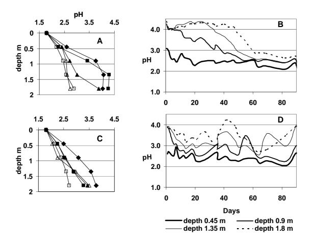
Figure 2. Discharge solution pH as a function of time: A & B, aerated; C & D, unaerated. ◆ 5 days; ■ 20 days; ▲ 50 days; □ 65 days; △ 85 days;
