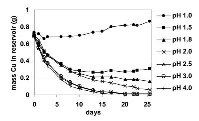
Figure 6. Mass of copper in column reservoirs maintained in the pH range 1.0 to 4.0.
