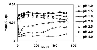
Figure 7. Mass of copper in leachates for flasks that contained 4 g pulverised ore and 0.012 g Cu as copper sulfate. The legend denotes the initial solution pH.
