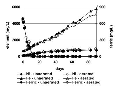
Figure 4. Nickel, total iron and ferric ion concentrations in column reservoir solutions.
