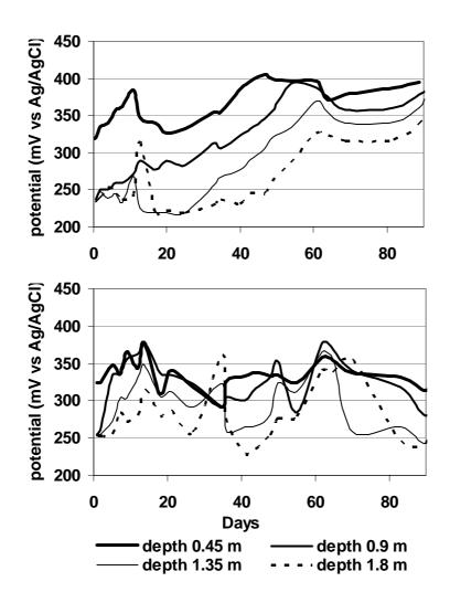
Figure 3. Redox potential of column discharge solutions: A, aerated and B, unaerated
