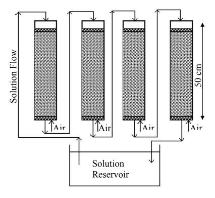
Figure 1. Schematic diagram showing the flow of synthetic leach solution and air through four columns operated in series. The four unaerated columns were set up without air inlets.
