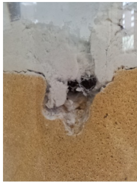
Fig. 7 Floating GCLs sample and air space under sample
