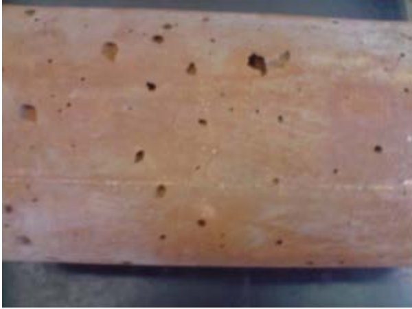
270 Figure 9. Typical cracks and colour change in the geopolymer concrete panels after fire 271 exposure
