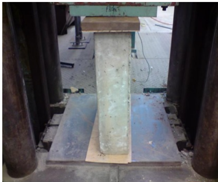
Figure 4. Post-fire compression test of a concrete panel
