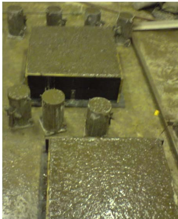
Figure 2. Casting of the geopolymer concrete test panels
