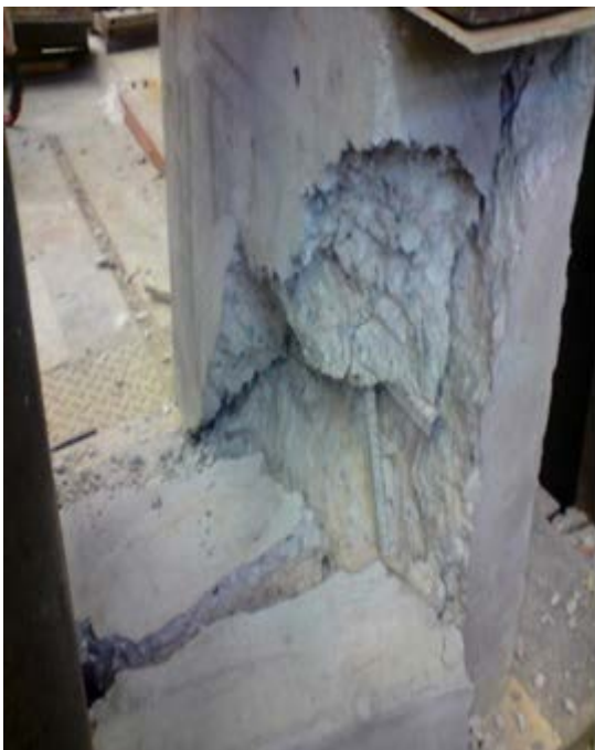
273 Figure 10(a). Failure of the 125 mm OPC concrete panel Figure 10(b). Failure of the 125 274 mm GPC panel
