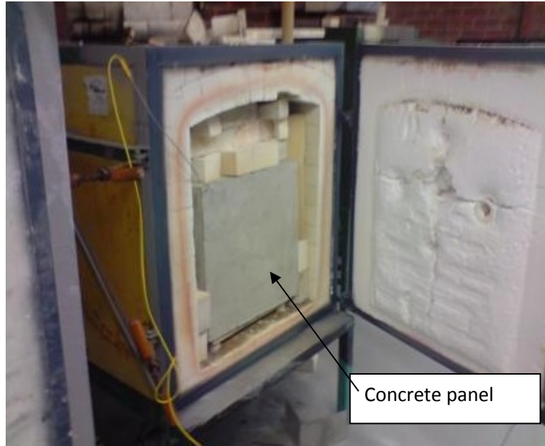
Figure 3. A concrete test panel set for fire exposure
