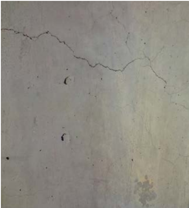
266 Figure 8(b). Typical cracks in the OPC concrete panels
