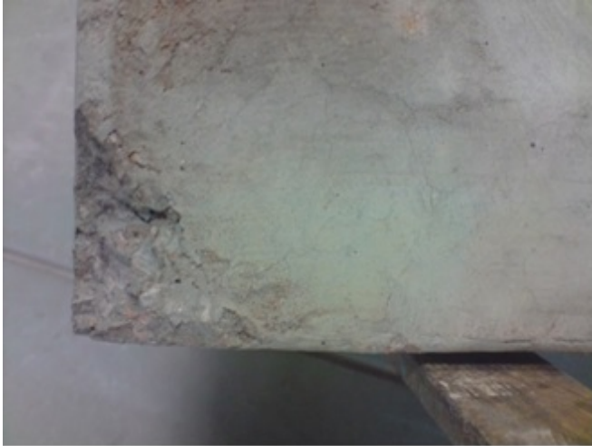
264 Figure 8(a). Corner spalling of the 125 mm thick OPC concrete panel
