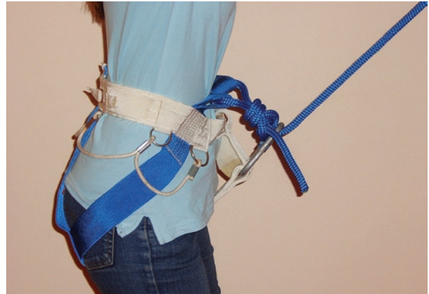
Figure 7. The Whillans Sit Harness, made by Troll. A significant feature was its ability to be worn over a wide range of thicknesses of clothing (in part due to the way the rope was attached).
