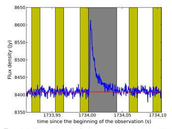
**Figure 1.** Dedispersed time series for the strongest giant pulse in the MWA data. The yellow (lighter) portions were used to estimate the off-pulse baseline shown by the red line. The gray (darker) area is the region that was integrated over to measure the total pulse energy. The plot spans 180 ms and has a time resolution of 400  $\mu$ s.
