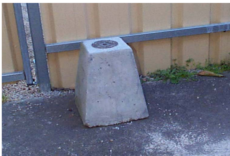
Figure 3. Pre-cast PSM with plaque glued to the top. The plaque will be situated just below the surface after the PSM is installed in the ground, with the raised centre of the plaque the measuring point.
