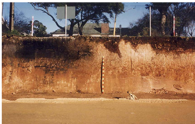
Figure 1. Cross-section of excavation in Adelaide metropolitan area revealing light coloured Keswick Clay pushing up through the surface soil to form gilgai (from Sheard and Bowman, 1994).
