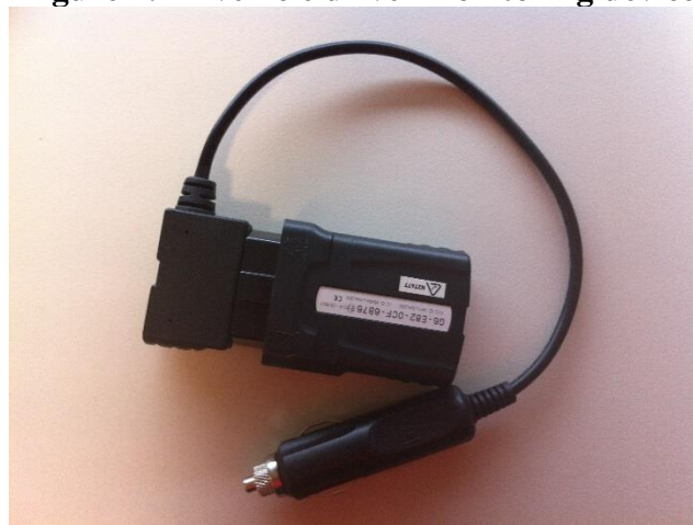
192 Figure 1: In-vehicle driver monitoring device
