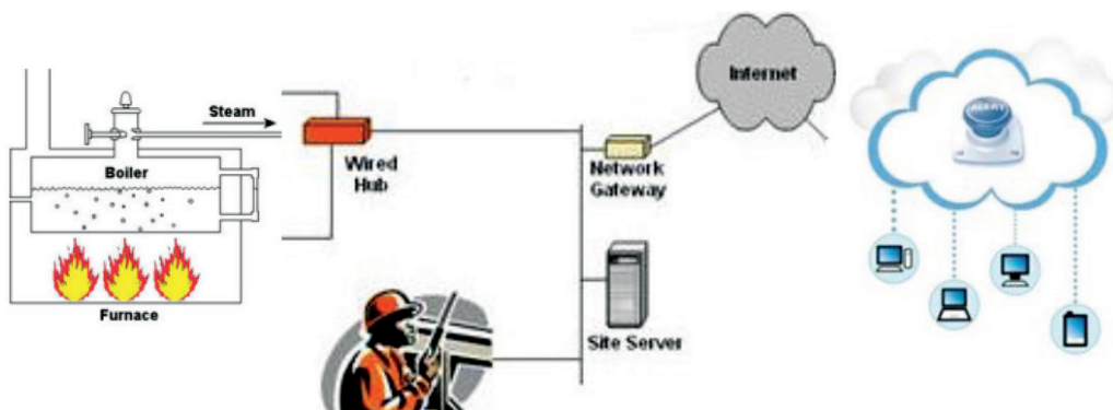
Fig.3: An improved interface monitoring system
