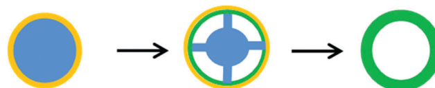
Fig. 9 Hollowing by the Kirkendall effect.
