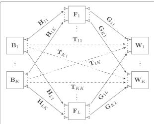
Figure 1 Block diagram of an interference MIMO relay system.
