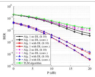
**Figure 3** Example 1: BER versus *P* at different number of iterations.
