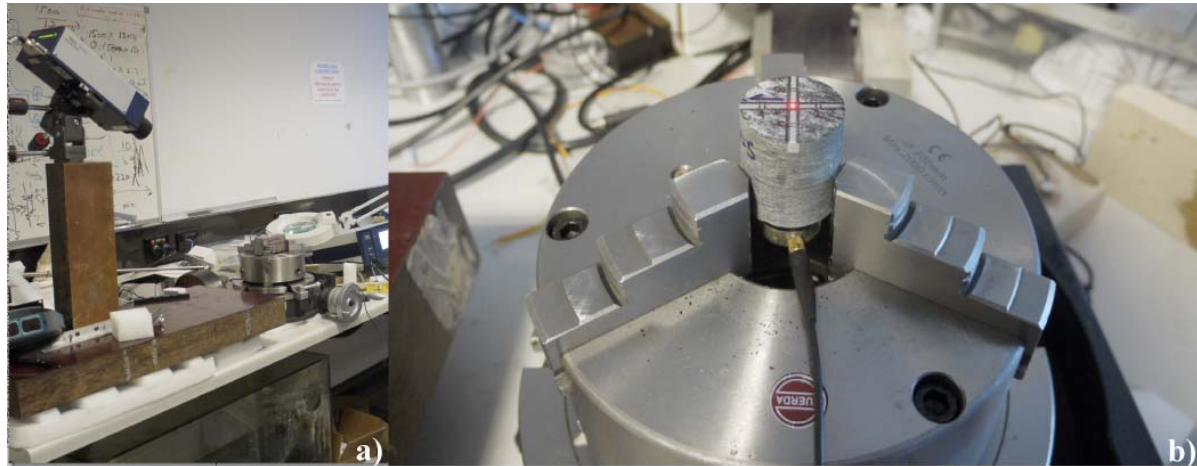
Figure 2 (a) Laser interferometer device and (b) an example of sample set-up used to study anisotropic nature of some of the samples taken from a major deformation zone.
