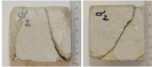
Figure 3 Typical failure planes in the sandstone cubes after true triaxial tests, showing the growth of failure planes parallel to \sigma_2 . Here \sigma_1 is acting axially and \sigma_3 acts in lateral direction.
