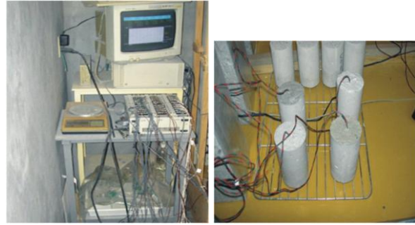
Fig. 4: Instrumentation for free shrinkage test The outer radius of the mortar ring is 190 mm therefore its thickness is 40 mm. Then radial drying of ring specimens was conducted in the laboratory atmosphere with RH of 60% and at 20°C. Drying was only allowed from the outer circumferential surface. The large depth-to-thickness ratio was chosen to provide uniform drying across the thickness [4] .
