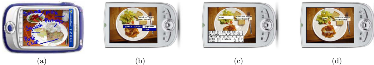
Figure 2. Additional input devices and labels for use with mobile device food record (a) Using stylus to hand write notes to label food items in a digital picture of a meal, (b) Using the an onscreen tree method to label food items in a digital picture of a meal, (c) Using an onscreen keyboard to search for a food item from the database and (d) A labeled meal and not shown are the secondary prompts for dressing on salad and spread on bread.
