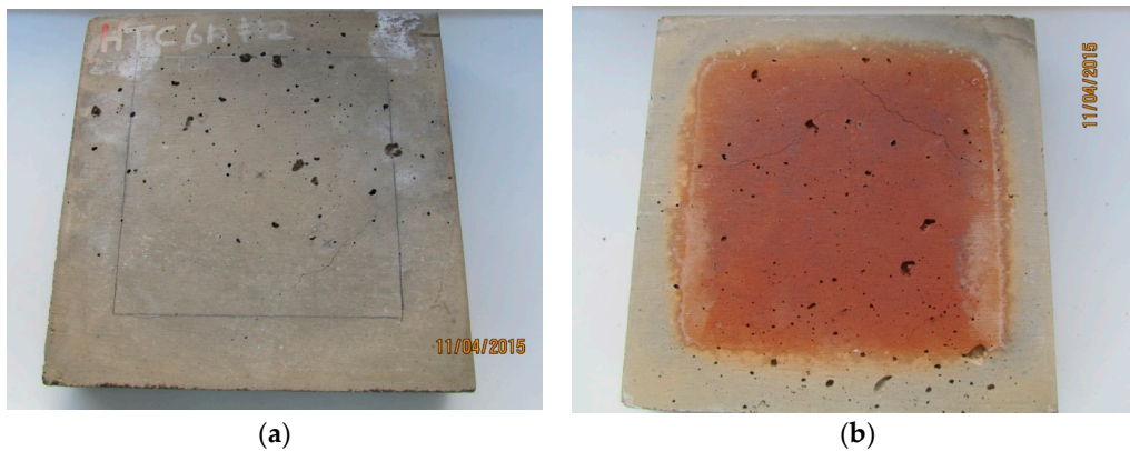
Figure 11. HTC 6A fire test images: (a) HTC 6A cold side after fire test; (b) HTC 6A hot side after fire test showing few minor cracks.
