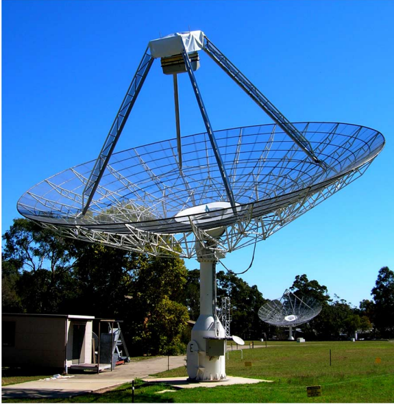
Fig. 2. The two dish prototype radiotelescope located in Sydney; the east antenna in the foreground is fitted with the FPA and the west antenna in the background with a single horn.
