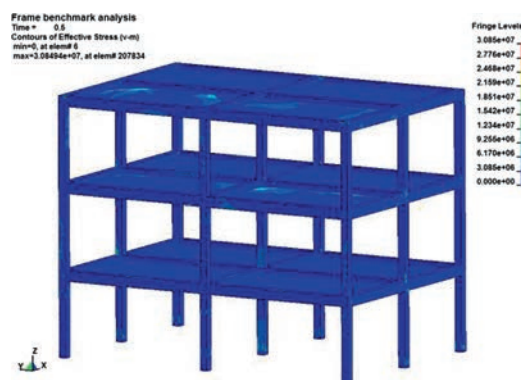
Figure 4. Structural response at 0.5 sec
