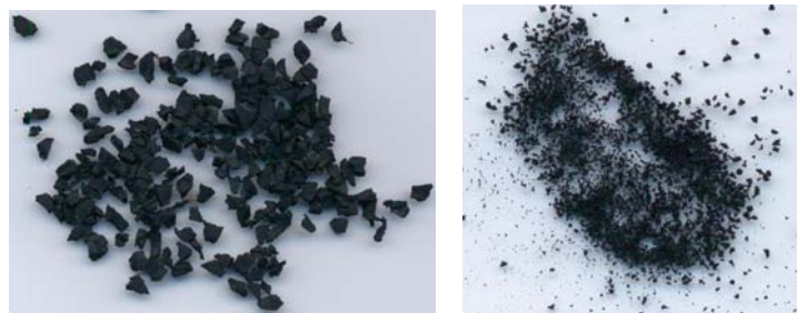
Fig. 3 Photographs of the 4 mm tire grains (left) and 750 \mu\text{m} tire powder (right)
