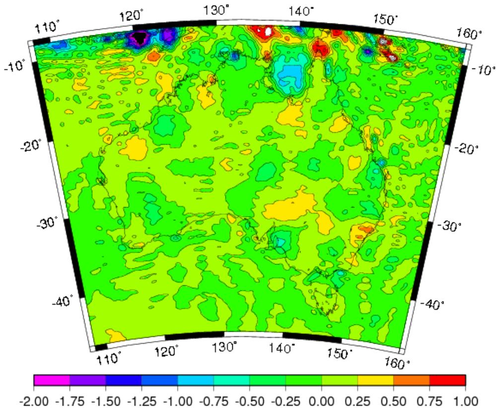
**Figure 2** Differences between EGM96 and EIGEN-GL04C quasigeoid heights to degree 360 (~55 km resolution) over the AUSGeoid98 area (Units in metres; Lambert projection). This is identical to the differences between AUSGeoid98 and AG98+GL04C.
