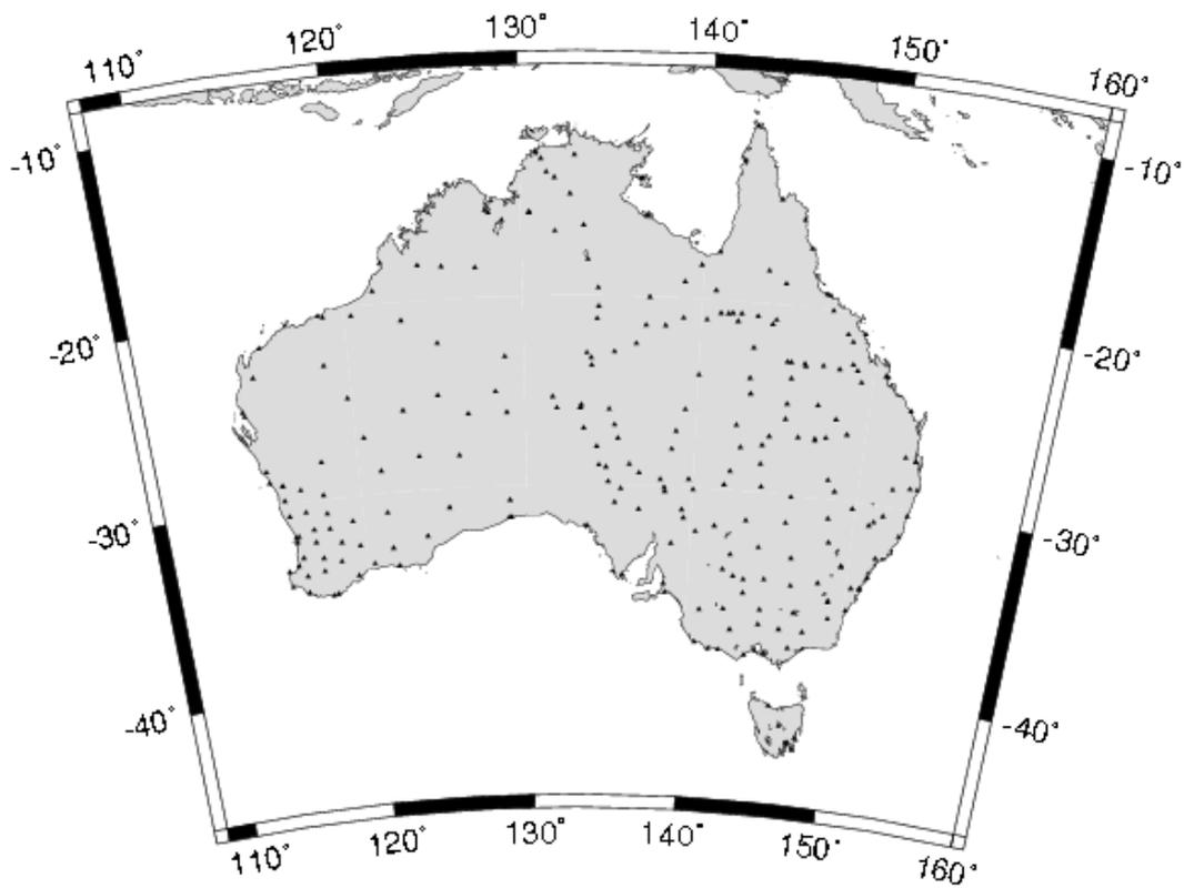
**Figure 4** Coverage of the 254 GPS-levelling points (Lambert projection).
