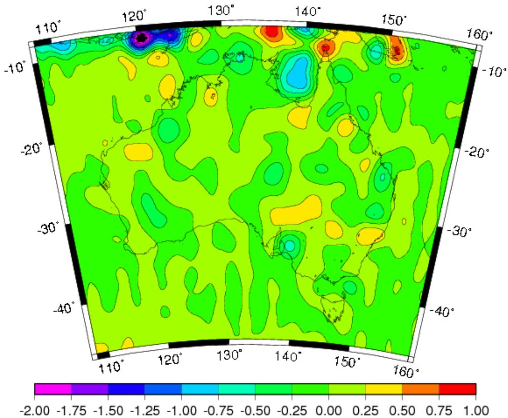
**Figure 1** Differences between EGM96 and GGM02C quasigeoid heights to degree 200 (~100 km resolution) over the AUSGeoid98 area (Units in metres; Lambert projection). This is identical to the differences between AUSGeoid98 and AG98+GGM02C.
