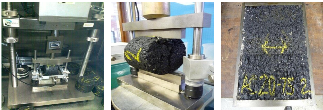
(a) Dynamic creep test
