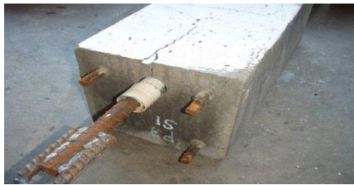
Figure 2(a). Failure of Geopolymer Concrete Specimen
