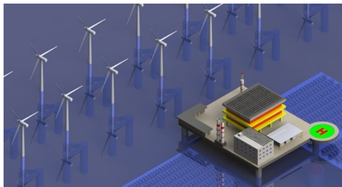
Figure 8. Multiple units of wind turbines and solar panels installed on offshore platform (conceptual design from [8])
