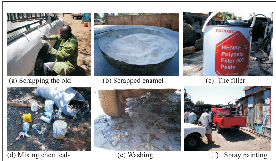
Figure 5: The spray painting process and wastes
