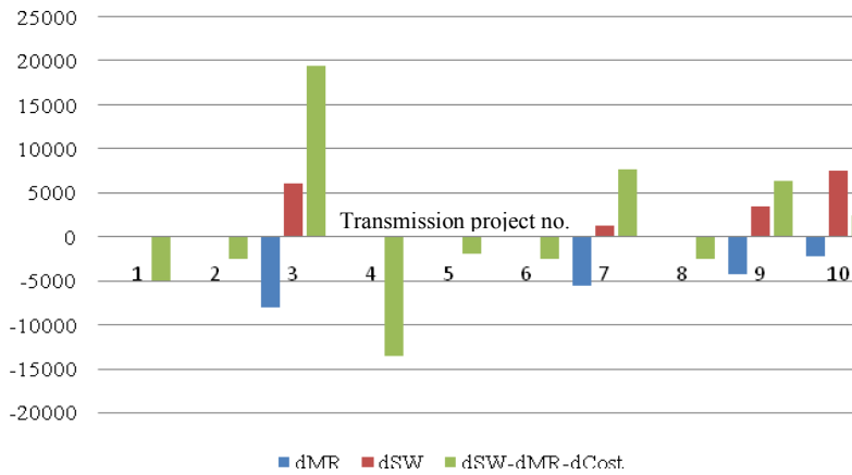
Figure 4, Effect of transmission projects on SS and MR during iteration 1 of the Three-stage Model
