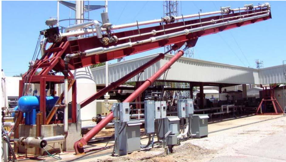
Figure 2 – The drilling section of Advance Cuttings Transport Facilities (ACTF) of Tulsa University at inclination of 25 degrees (Miska et al., 2004)
