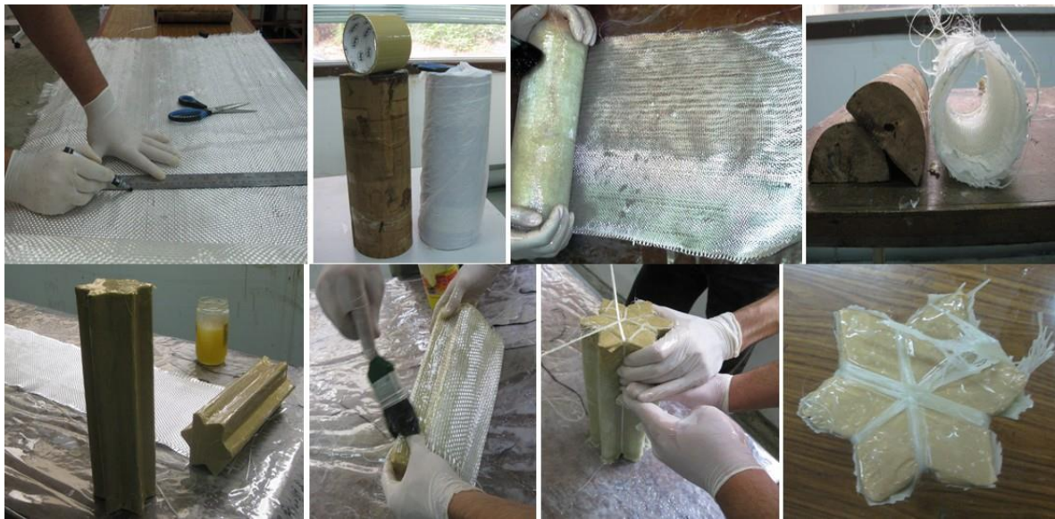
Figure 4. Hand lay-up method.
