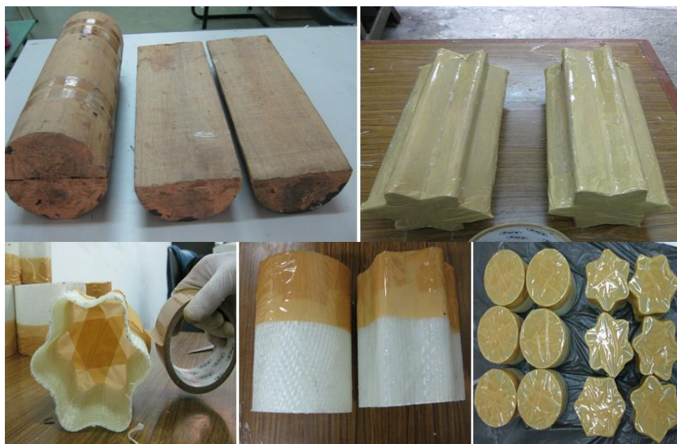
Figure 3. Circular and corrugated wooden mandrels. Preparing specimens to add the fillers.
