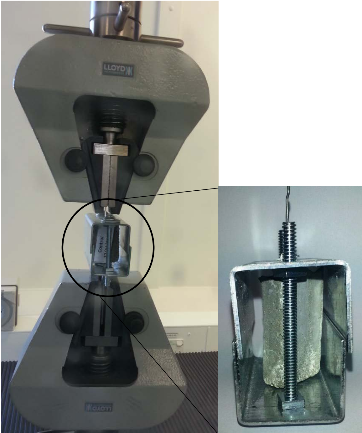
2 Fig. 3 Test setup of pull-out specimen. (Close-up shows the pull-out specimen inside the steel tube 3 and the fibre passed through the top circular hole)
