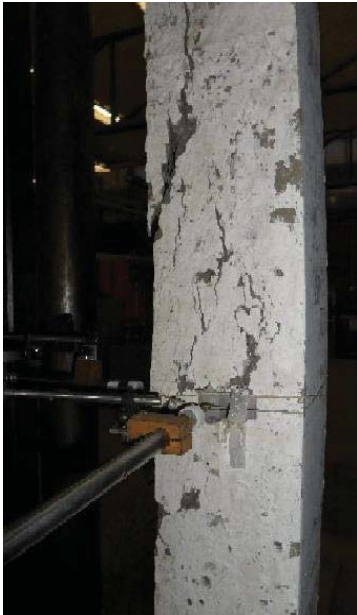
(b) Crushing on compression sides
