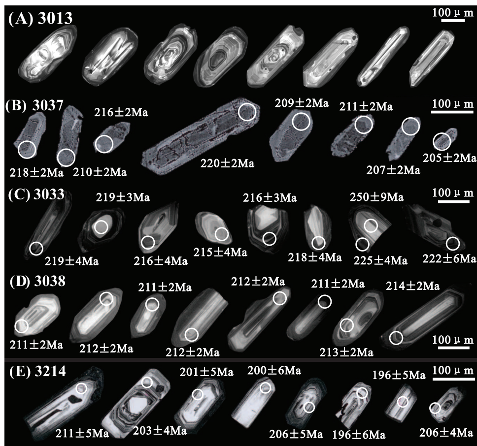
Fig. 3. Cathodoluminescence (CL) images of selected dated zircon grains from samples #3013, #3033, #3038 and #3214, and scanning electron microscope backscatter (BSE) images of sample #3037 from the granites in the Chinese Altai. Analyzed spots are circled, and numbers refer to U-Pb ages presented in table 1.
