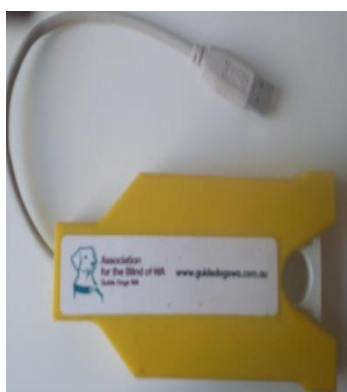
Fig 1. Designed USB cartridge for Blind or limited mobility people
