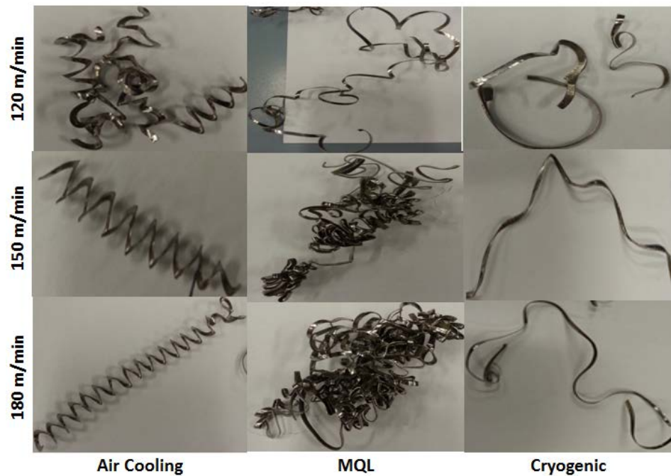
Figure 8. Chip formation for varying cutting speeds and cooling methods.
