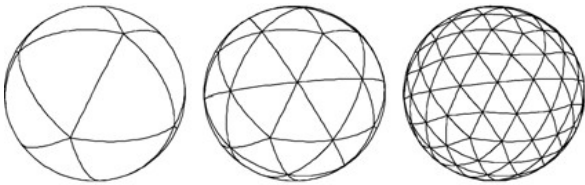
Figure 10: Spherical meshes subdivision. The subdivided meshes are used for sampling [31]
