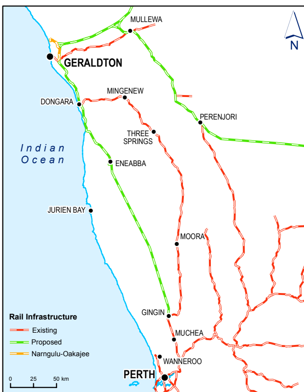
Figure 6.2: Existing and proposed rail infrastructure
