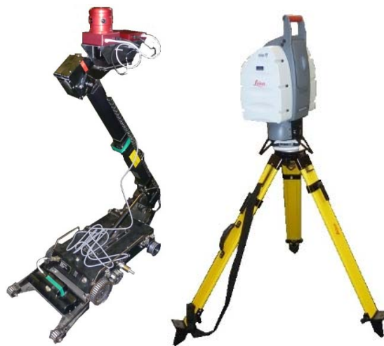
Figure 1. (Left) The Point Grey Ladybug Omnidirectional Camera mounted on the Cyclops robotic platform. (Right) The Leica ScanStation on its tripod.
