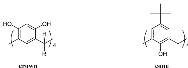
Figure 9. “Simplified” depictions of the resorcinarene crown conformation shown with “all axial” alkyl groups and the calixarene cone conformation.
