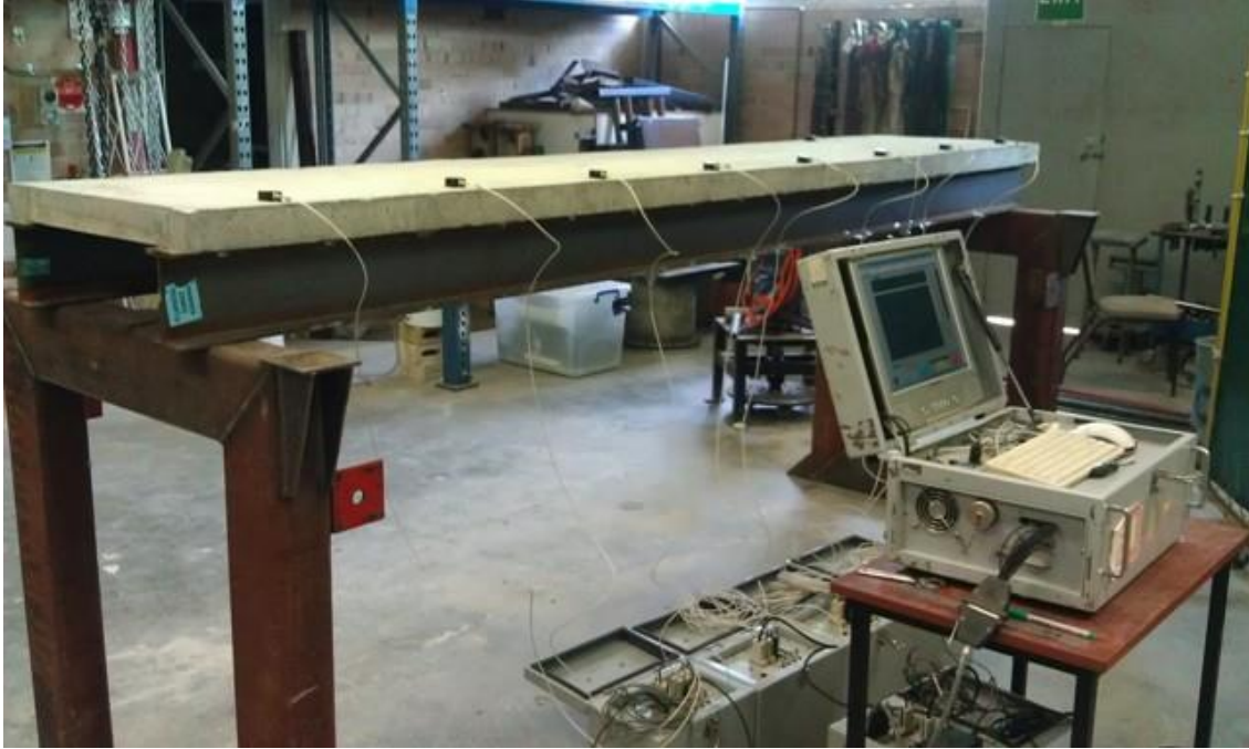
Figure 11 - Experimental test setup of the slab-on-girder structure
